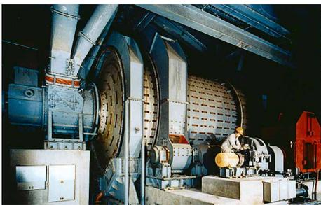
At the Dezhou Shandong Huaneng Power Development Co. Ltd. power plant in China, sealing air is used to contain hot exhaust air laden with coal dust in the neck of a coal mill. The ideal solution: An **Espey WD200/500**. Operating conditions:  $p = 1.08 \text{ bar}$  (15.66 PSI);  $t = 110 \text{ °C}$  (230 °F);  $n = 15.8 \text{ min}^{-1}$ .
