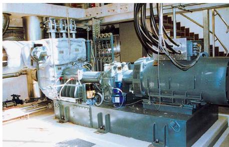
Hot steam has to be contained in a turbine at the Vapo Oy Pellet power station in Finland. An **Espey WKA400** carbon floating ring seal with steam and condensate leakage drain is used in this application. Operating conditions:  $p = 23 \text{ bar}$  (344 PSI);  $t = 495 \text{ °C}$  (923 °F);  $n = 8,200 \text{ min}^{-1}$ .
