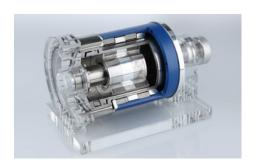
EagleBurgmann has designed a new high performance magnetic coupling type NMB 22P-10R-65-ND2. This is installed in a multistage vertical can pump of an ethylene cracker unit in a German refinery. p = ... 65 bar (943 PSI); t = -32... +40 °C (-26 °F ... +104 °F);  $n = 2,980 \text{ min}^{-1}$ ; drive power: 315 kW direct start; design torque: >1,700 Nm. Media: hydrocarbons C2+C4.
