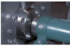
In a cracking unit in the United States a compressor is sealed by EagleBurgmann Espey carbon floating ring seals type WD200 and WDKS. Operating conditions: p = ... 5 bar (73 PSI); t = 75 °C  $(167 \text{ °F}); n = 3,000 \text{ min}^{-1}; d1 = 55 \text{ mm } (2.17").$ Medium: cracked process gas (containing dust).
