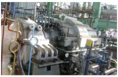
Bhel compressor in the delayed coker unit of the Panipat refinery run by the Indian Oil Corporation Ltd. The machine is equipped with EagleBurgmann **DGS20.1/200** tandem gas seals and a **diaphragm coupling**. Operating conditions: p=6 barg (87 PSIG); t=150 °C (302 °F); n=8,909 min<sup>-1</sup>; t=180 mm (7.09"). Medium: flue gas.
