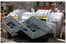
EagleBurgmann **high-end standpipe expansion joint** installed in a refinery in Texas, USA. Operating conditions: p = ... 6.89 bar (100 PSI); t = 510 °C (950 °F); d = 1,170 mm (46"). Medium: flue gas.
