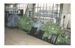
Coking oven gas compressor (Mannesmann Demag) at Wintershall AG, Lingen. Originally equipped with labyrinth seals, the turbine-driven single-shaft radial compressor has been converted to EagleBurgmann dual **DGS** seals and a buffer gas supply system. Operating conditions: p=5.6 barg (81 PSIG);  $n=12,800 \text{ min}^{-1}$ ; d1=134.8 mm (5.3"). Medium: gas with  $H_2S$  content.
