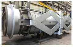
EagleBurgmann provided a large sized universal spent catalyst standpipe expansion joint for a refinery in Texas, USA. Operating conditions: p = ... 3.79 barg (55 PSIG); t = 732 °C (1,350 °F);d = 1,500 mm (59").
