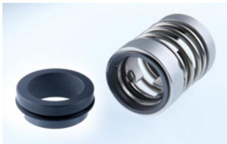
**HA211** type mechanical seals operate in the fiberization process of the mechanical pulp production at Nippon Paper in Japan to provide secure sealing of white water. Operating conditions:  $p = 1 \text{ bar (15 PSI)}$ ,  $t = 30 \text{ }^\circ\text{C (86 }^\circ\text{F)}$ ,  $n = 1,450 \text{ min}^{-1}$ .
