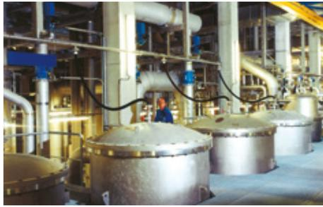
At UPM Kymmene Shotton in England, nine Voith pressure screens in waste paper treatment are being used successfully with EagleBurgmann **HR-D** type double cartridge seals. Medium to be sealed: Pulp fibers 1.5 ... 4 % abs. dry and water,  $p = 8 \text{ bar (116 PSI)}$ ,  $t = \text{max. } 40 \text{ }^\circ\text{C (104 }^\circ\text{F)}$ .
