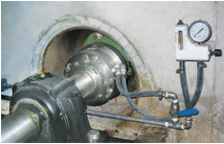
Chest agitators at Sappi in Lanaken/Belgium were retrofitted to EagleBurgmann **HGH** type semi-split mechanical seals. Since then, product leakage has been drastically reduced and plant availability has noticeably increased. Operating conditions:  $p = 0.5 \text{ bar (7.25 PSI)}$ ,  $t = 20 \text{ }^\circ\text{C} \dots 40 \text{ }^\circ\text{C}$  ( $68 \text{ }^\circ\text{F} \dots 104 \text{ }^\circ\text{F}$ ),  $n = 300 \text{ min}^{-1}$ .
