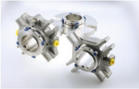
A successful seal type for the entire plant: Over 250 standardized EagleBurgmann **Cartex** cartridge seals are installed in pulp pumps and in the pumps of the chemical sector at the Swedish Iggesund Holmen paper and pulp mill. Operating conditions:  $p = 12 \dots 25 \text{ bar (174} \dots 363 \text{ PSI)}$ ,  $t = -40 \text{ }^\circ\text{C} \dots +220 \text{ }^\circ\text{C}$  ( $-40 \text{ }^\circ\text{F} \dots +428 \text{ }^\circ\text{F}$ ),  $n = 1,660 \text{ min}^{-1}$ .
