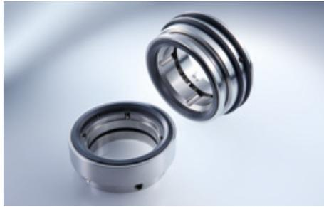
For the reliable sealing of black liquor, **L9UC** type mechanical seals are used at Nagayo Paper in Japan. Operating conditions:  $p = 3 \text{ bar (44 PSI)}$ ,  $t = 85 \text{ }^\circ\text{C (185 }^\circ\text{F)}$ ,  $n = 1,750 \text{ min}^{-1}$ .
