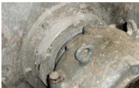
A horizontally arranged machine shaft is sealed by an Espey **E-WDKS205** type carbon floating ring seal at Norske Skog Saugbrugs in Norway. Operating conditions:  $t = 40 \text{ }^\circ\text{C} \dots 50 \text{ }^\circ\text{C (104 }^\circ\text{F} \dots 122 \text{ }^\circ\text{F)}$ ,  $n = 11 \dots 15 \text{ min}^{-1}$ .
