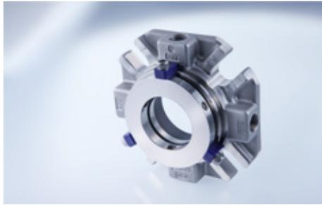
An EagleBurgmann **MA291** type mechanical seal operates at the Hakuetsu Paper in Nayo, Japan and seals the white water of the paper machine. Operating conditions:  $p = 2 \text{ bar (29 PSI)}$ ,  $t = 100 \text{ }^\circ\text{C (212 }^\circ\text{F)}$ ,  $n = 1,470 \text{ min}^{-1}$ .
