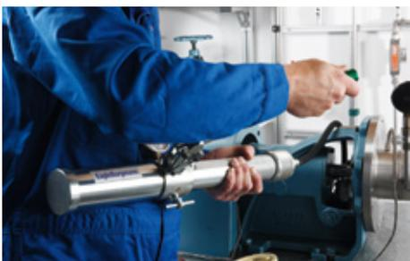
EagleBurgmann **Burajet SF6335** and **Burajet 8032SCW** type compression packings are installed in Andritz refiners as shaft seals at the Mexican paper factory Copamex Papelara de Chihuahua. Operating conditions:  $p = \text{max. } 16 \text{ bar (232 PSI)}$ ,  $t = 200 \text{ }^\circ\text{C (392 }^\circ\text{F)}$ .
