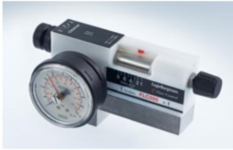
The EagleBurgmann **FLC200** flow control unit is used for all dual seals of the Stora Enso Skutskär paper mill in Sweden in order to adjust the volume of supplied water as needed. Safe operation of the seals is thus ensured. Operating conditions:  $p = 25$  bar (363 PSI),  $t = 85 \text{ }^\circ\text{C}$  (185  $^\circ\text{F}$ ).
